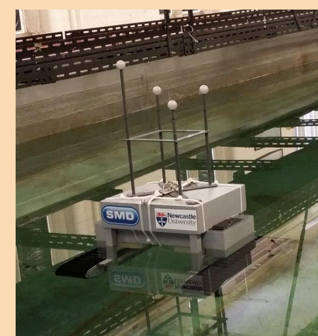
ROV model (scale ratio of 1:12)
